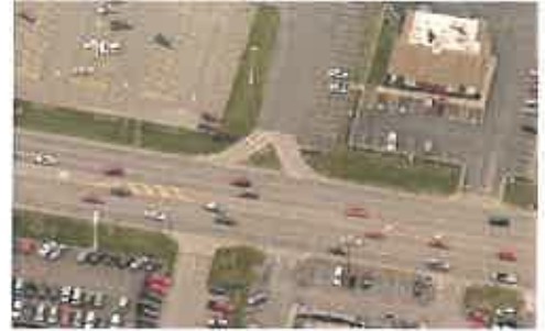
FIGURE 5: RIGHT-IN / RIGHT-OUT DRIVEWAY
